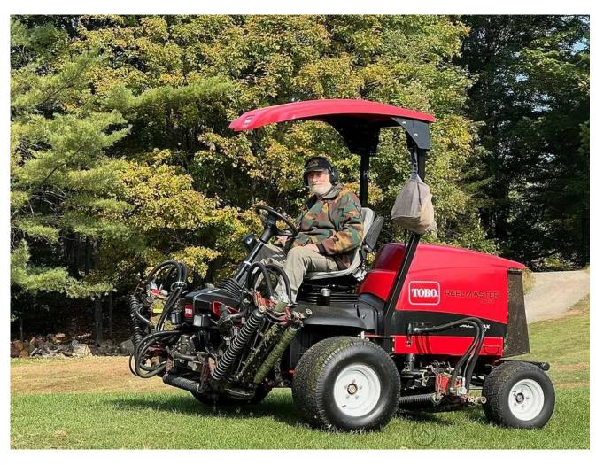
Terrific news! DCC fairways are about to make a giant leap forward with the acquisition of a "new to us" Toro dedicated ride-on fairway unit. This mower has the cutting units out in front of the operator, making it much easier to follow the same path on the cleanup. This results in remarkably improved definition between the fairway cut and the rough; in short, a much-improved course!
